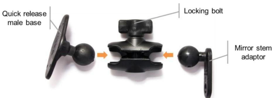
The scooter kit is made to be mounted on the mirror stem. The mirror needs to be undone at the base of its stem using the appropriate spanner. The mirror / pinchbolt mount will then usually be fitted on the threaded portion of the stem and re-assembled with it. Some mirror stems are not threaded and are fixed using a conical pressure bolt. If this is the case, alternative RAM® solutions must be investigated.
